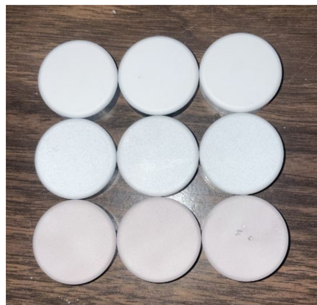
All 9 different indentation samples photographed from above with the alumina samples highest the yttria samples in the middle and the lanthanum zirconate samples at the bottom
