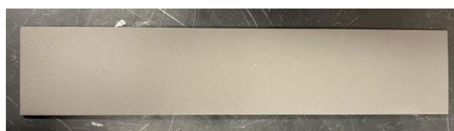
Uncoated machined aluminum 4-point bend sample used for test setup validation
